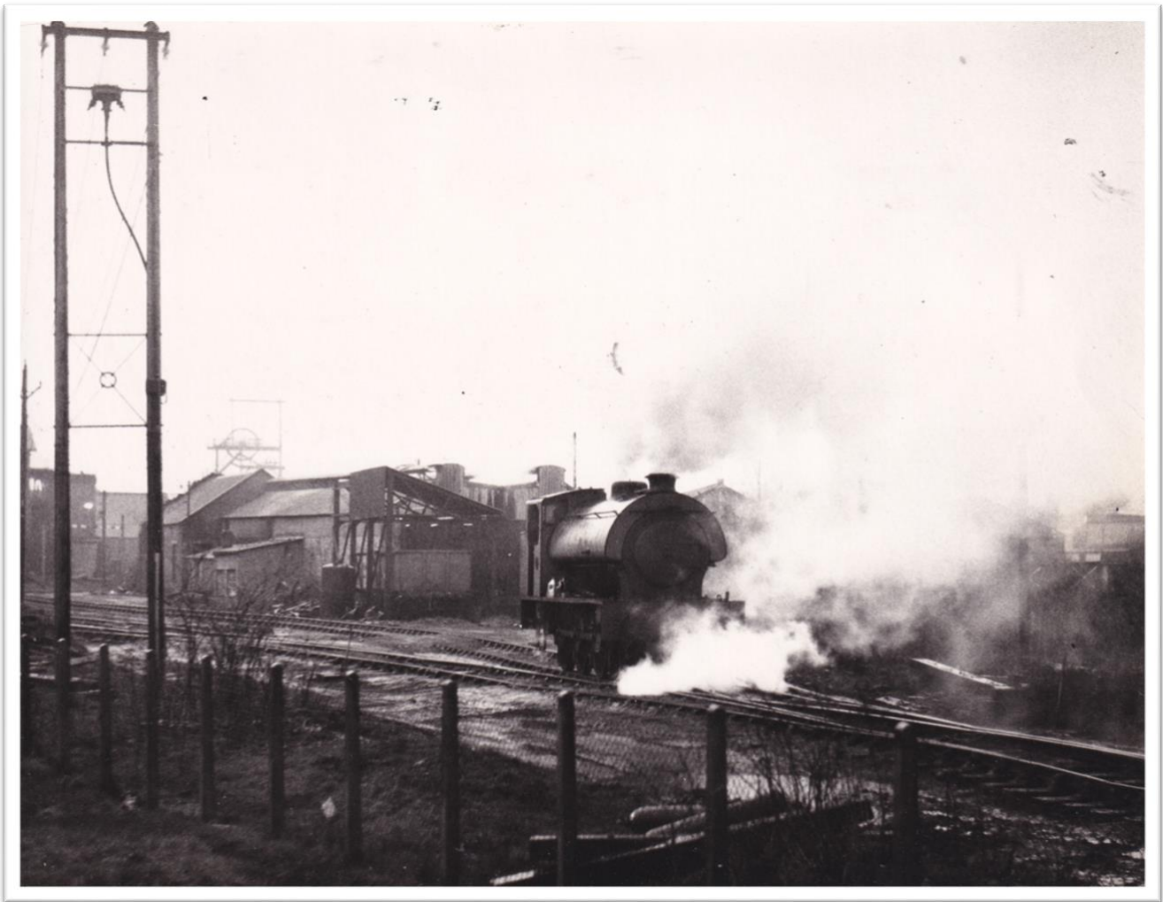
Robert Stephenson & Hawthorns 'Austerity' 0-6-0 saddle tank 'NCB No.8' (Works No. 7139 built in 1944) at Mountain Ash 'Phurnacite' works.
